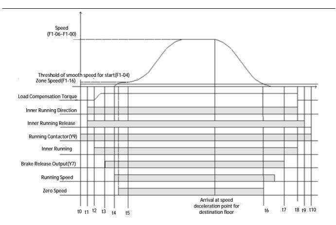
FIGURE 6.3 ELEVATOR TIMING DIAGRAM FOR NORMAL RUNNING
