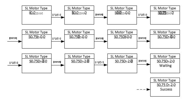
FIGURE 4.25 BLUE-LIGHT MACHINE INPUT FLOW CHART
