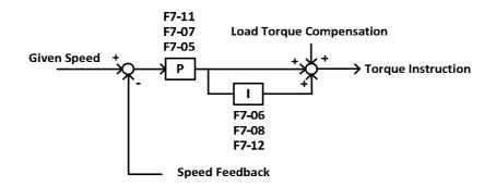
FIGURE 6.12 SPEED ADJUSTMENTS 2
