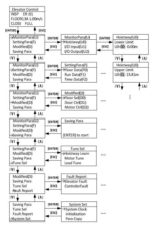
FIGURE 4.3 STRUCTURE FLOWCHART OF OPERATOR MENU
