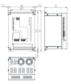
FIGURE 2.5 SHIELD TYPE EXTERIOR DIMENSION
