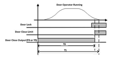
FIGURE 6.8 TIMING DIAGRAM FOR DOOR CLOSE
