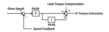
FIGURE 6.11 SPEED ADJUSTMENTS 1
