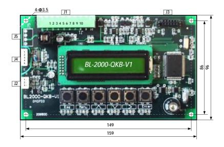
FIGURE 11.22 GROUP CONTROL BOARD BL2000-QKB-V1 SHAPE & DIMENSION
