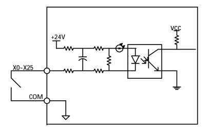
FIGURE 3.6 CONTACTOR SWITCH INPUT
