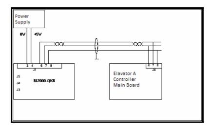
FIGURE 11.23 GROUP CONTROL BOARD BL2000-QKB-V1 INTERFACE CIRCUIT
