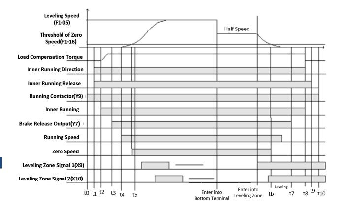
FIGURE 6.6 TIMING DIAGRAMS FOR RECALIBRATION RUNNING (SAME DEFINITION & SETTING WITH NORMAL RUNNING)
