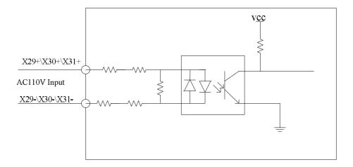
FIGURE 3.9 AC110V INPUT INTERFACE & CONNECTIONS
