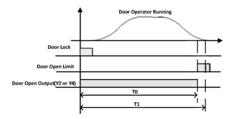
FIGURE 6.7 TIMING DIAGRAM FOR DOOR OPEN
