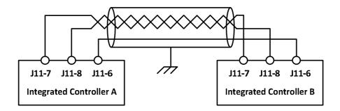
FIGURE 6.9 CONNECTION FOR DUPLEX CONTROL
