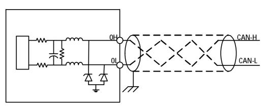
FIGURE 3.7 CAN COMM INTERFACE AND CONNECTION
