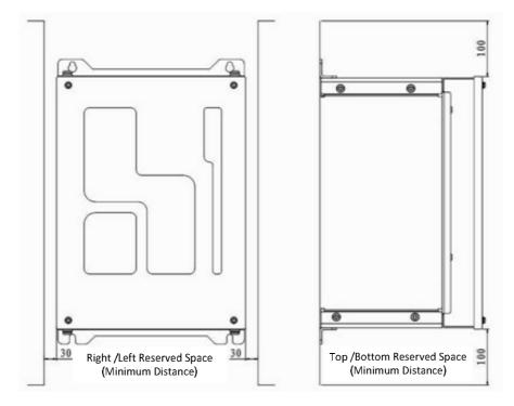
Figure 2.9 Driver Installation Orientations and Space
