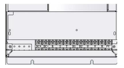
Figure 3.3 Terminal arrangements for main circuit
