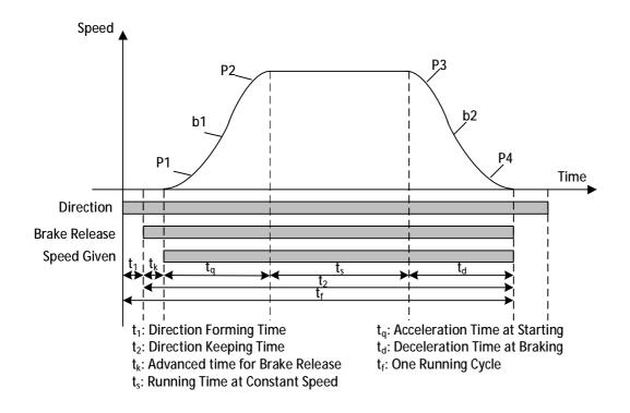
FIGURE 7.6 ELEVATOR RUNNING SPEED CURVE
