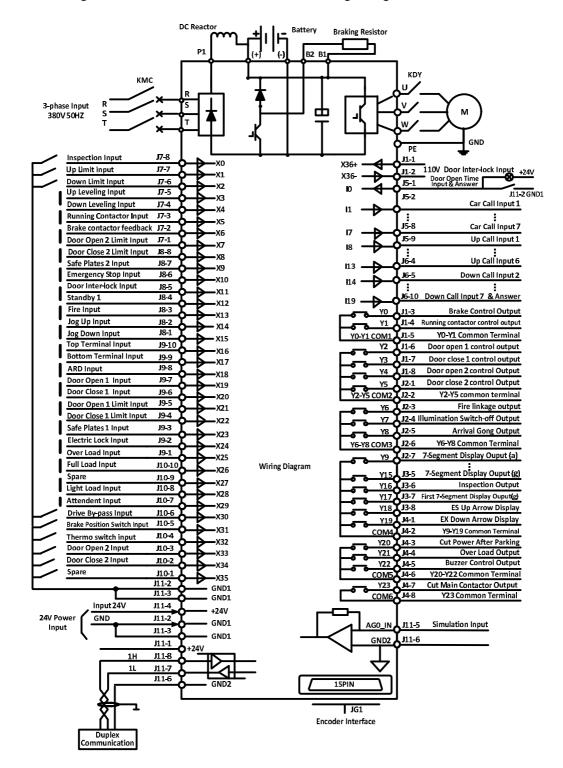
Figure 3.1 Therminal wiring Diagram for Elevator integrated controller
